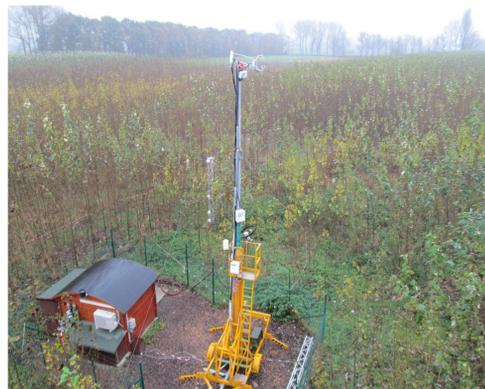
Fig. 1 Aerial view of the eddy covariance tower to monitor the GHG exchanges
