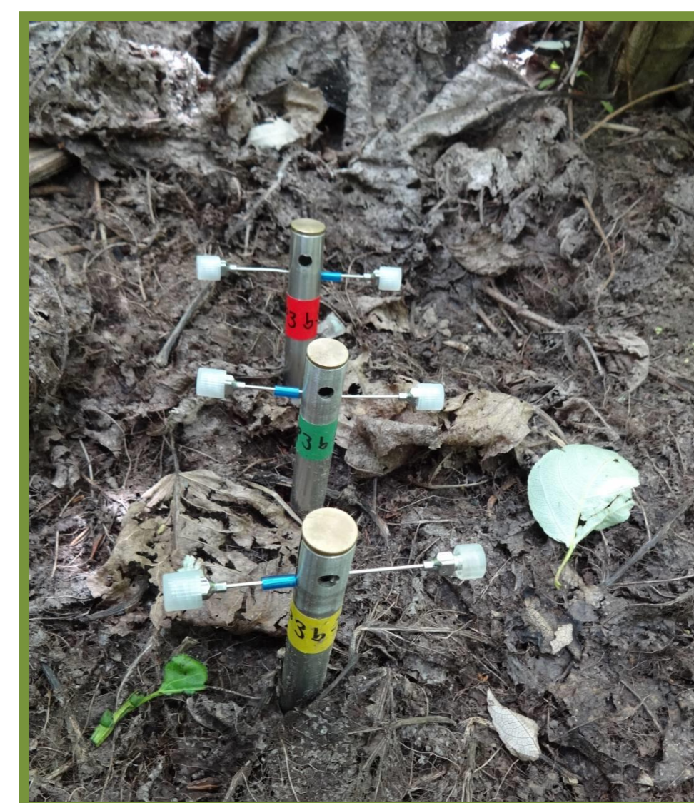
Soil gas samplers at 5, 15 and 50 cm depth (2).
